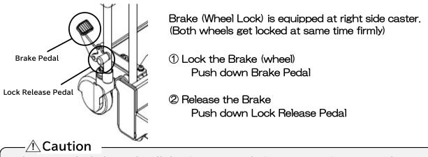
Make sure to lock the Brake all the time except during maneuvering. Or stacker may start to move all of a sudden and may result in accident.
