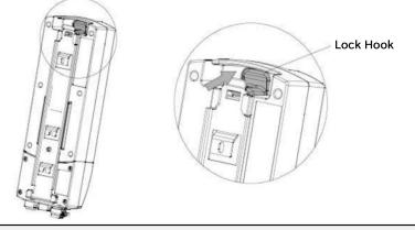
% Push Emergency Stop Switch and disconnect power before handling battery
